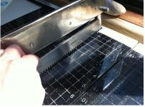
STEP 3: Remove cutting mats and make sure blade is flush with the base of the cutter.
