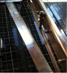
STEP 2: Align new blade into slot and lower handle so the blade slides up into the slot.
