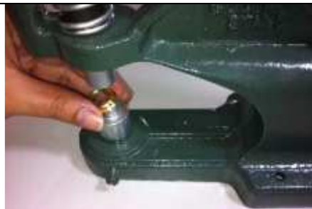
Step 1: Place the grommet on the bottom die.
