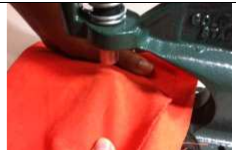
Step 2: Place the material on top of bottom die.
