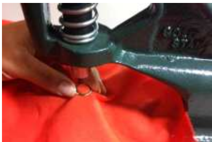
Step 3: Place the washer on the material. Lower handle to line up everything carefully.
