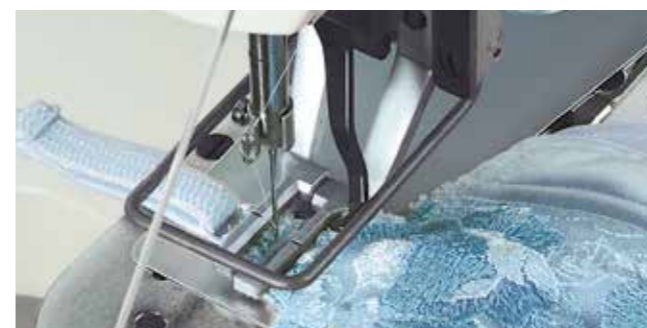
F type (Attaching the shoulder straps to brassier) * Presser foot for vertical bartacking is supplied with the unit as an accessory.
