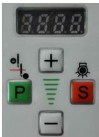
P, S keys for setting parameters or other functions;
