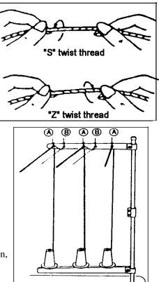
Note: Pressing the upper thread loosening button shown in the figure below opens the saucer of the upper thread tension adjuster, and the upper thread can easily pulled out.
