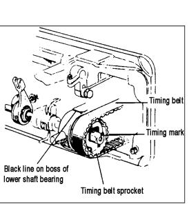
line with the black line on the boss of lower shaft bearing.
