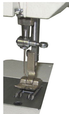
Closeup of needle adjusted to left position.
