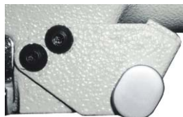
Push Button Reverse, Automatic Backtack Button conveniently located to the right of the needle
